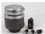
PL-002A Hydraulic Motor Pump *Model 5L: 65kg/cm 2 , 0.7/0.55l/min *Model 7.5L: 60kg/cm 2 , 1.1/0.9l/min *Model 10L: 50kg/cm 2 , 1.4/1.2l/min
