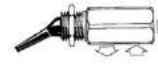
PL-328 Toggle Routing Valve *2-way routing, 1 input, 2 output *Panel-Mounting 15/32-32 hex nuts *For air or water *Gray color
