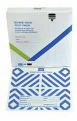
The test pack consists of a series of air removal and steam penetration barriers. Single use test packs are designed for validation in sterilization process in the sterilization process.
