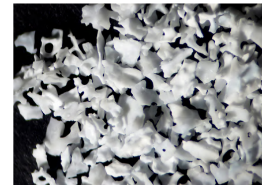
Company D Porous nature damaged The porous shape seems to be damaged in the production process
