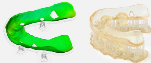
Full Arch Edentulous Surgical Guide Surgical Guide Resin, at 100µm Layer Height
