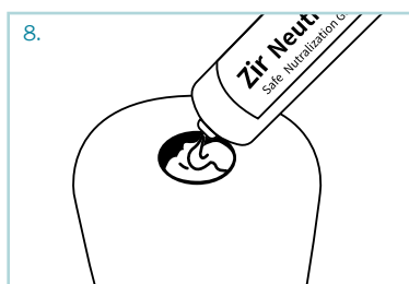
Apply Zir Neutralization Gel to the top of the Safe Shell (1) to close the injection port.
