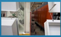
Then the process of treating and painting with epoxy powder coating is done by electrostatic method with a global RAL color code
