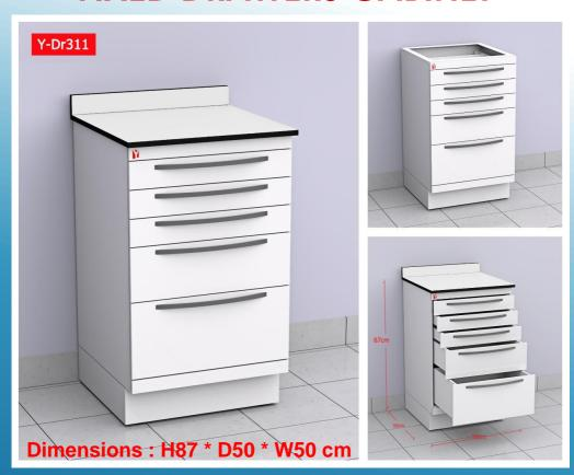
Fixed Drawers Cabinet with 5 drawers (three H1, one H2 & one H3) drawers. Made entirely of double layers galvanized steel sheet and electrostatically coated with epoxy powder
