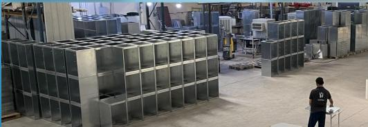
ALYARMUK Cabinets are designed to carry - safely - 250 kg / m2. The cabinet body is made of an integral part of galvanized steel sheets without welding, without joints and double-walled sides to increase durability, avoid weak joints, and ensure complete surface treatment and coating.
