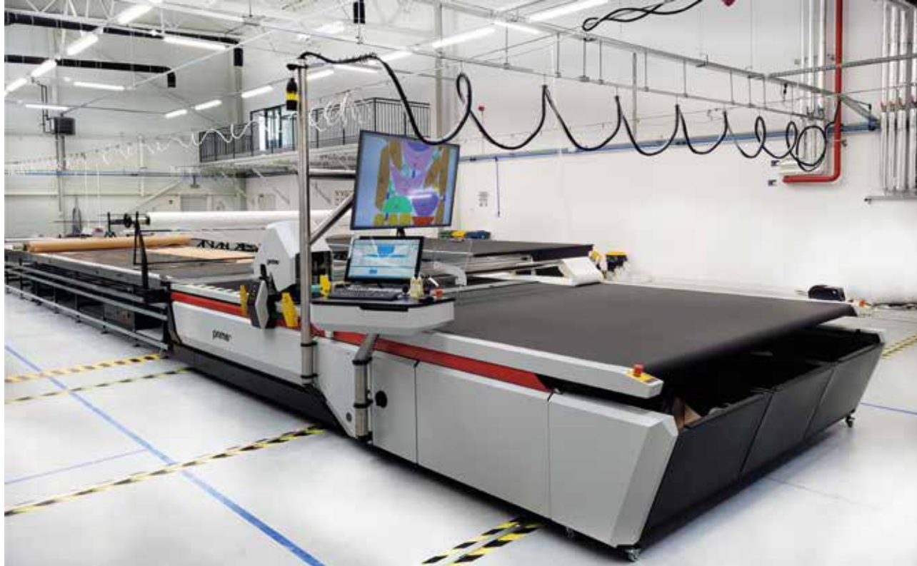
Prime.5 Multi-ply cutting system for textiles up to 5cm after vacuum
