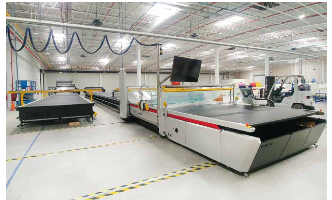
Prime.9 Multi-ply cutting system for textiles up to 9cm after vacuum
