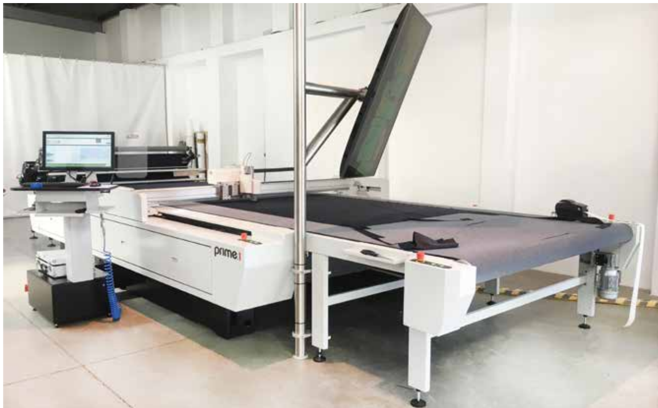
Prime.1 Single-ply cutting system for textiles
