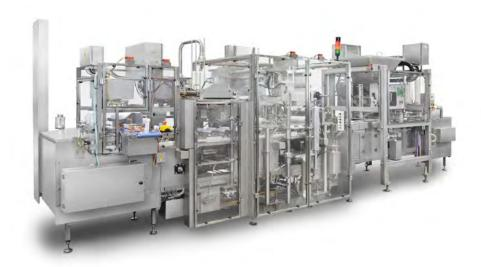
Highly flexible bar transport for quick format changes by push-button without time-consuming changes of format plates Absolute flexibility and optimized production times due to our unique patented bar transport.
