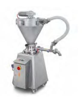
The EmulsiCut operates by rotor-stator-system. The cutting head rotates with a motor speed of 3000 rpm inside of the cutting ring, which defines the clearance between 11 and 0.2 mm. By a double cutting tool of different clearances, multiple cutting operations can be carried out in one step.
