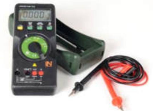
Multimeter with optical data interface for display via a virtual instrument on a PC.
