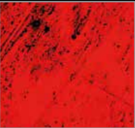
Test sample-Ceramir CAD/CAM BLOCKs no biofilm formation following exposure to bacteria.
