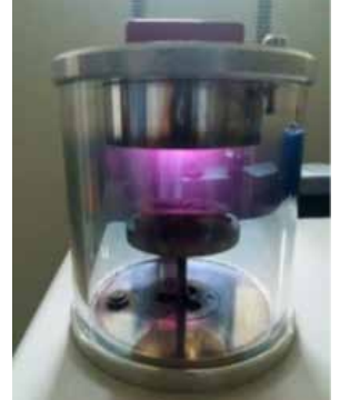
Metal coating chamber. (Magnetron Sputter Coater) JEOL JFC – 1200.
