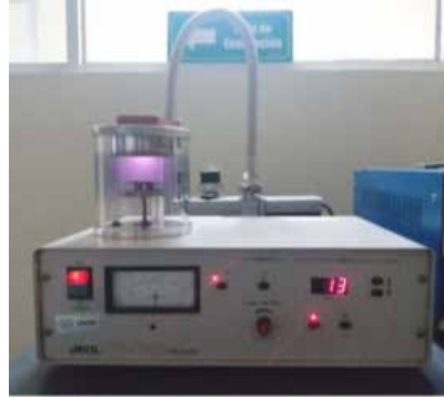
Metal coating chamber. (Magnetron Sputter Coater) JEOL JFC – 1200.
