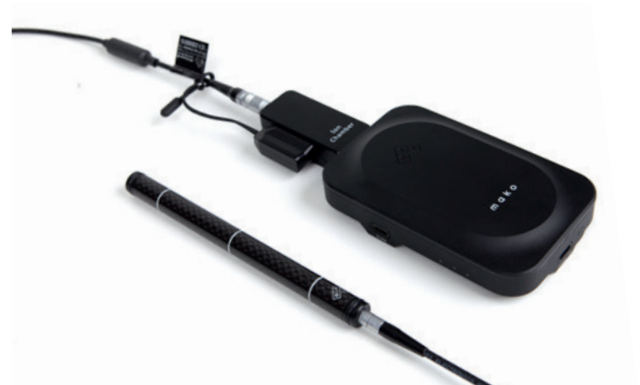
Mako Base Unit with Ion Chamber Module docked, and CT Ion Chamber attached.
