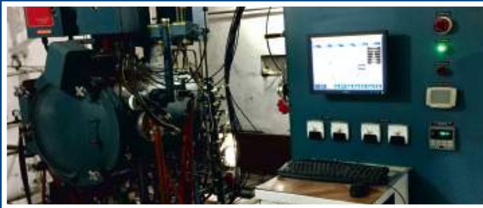
Vacuum Sintering Furnace made in USA
