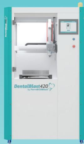
with titanium powder, aluminium oxide, calcium phosphate or ceramic. It can automatically process 420 implants in less than 4 hours, all while ensuring complete repeatability and the highest possible quality.
