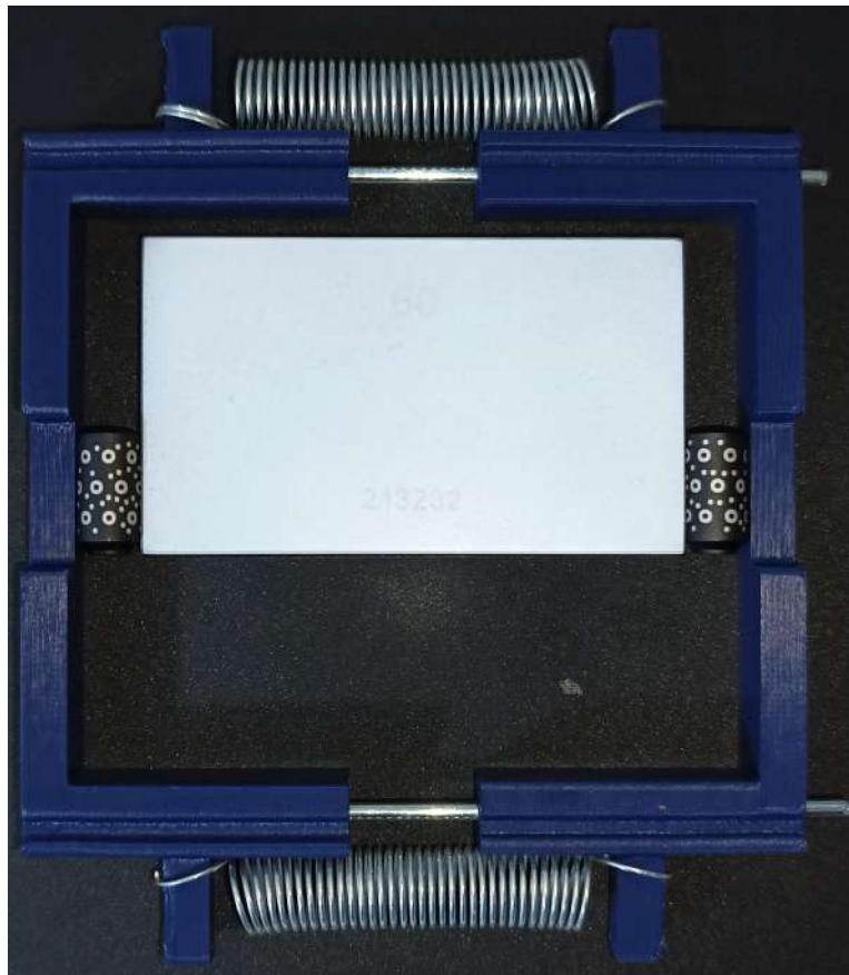
Figure 2: Posts pushed against a calibration block of known width, used to measure absolute accuracy.
