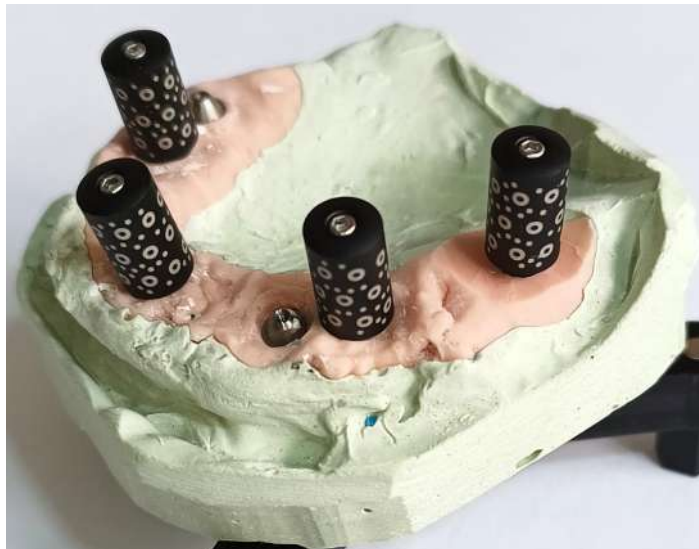
Figure 1: A stone cast model with 6 abutments embedded, used to measure the repeatability of post scanning measurements.
