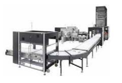
Gondola storage can increase the efficiency of a plant. A complete system from a single source, with all interfaces clarified and the focus placed on smooth, problem-free production. A row aligner with pullnose ensures an adjusted product flow after the pouring line. Premium packaging is provided by three LTM-DUO machines with an open fold on the first station, optimized for alternative packaging materials.
