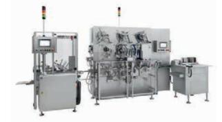
Line combination consisting of the GWS-M fold wrapping machine for packaging single chewing gum sticks in aluminum-backed foil and band wrap, subsequent grouping and production of a traditional chewing gum pack. The machine is directly connected to a multipack cartoning machine in order to manufacture a ready-to-sell display carton. Your system solution: our compact entry-level variant in the medium-speed range.
