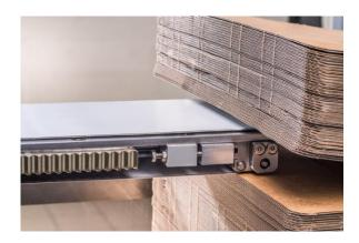
A clever solution: The redesigned vertical magazine can accommodate blanks of many different sizes.
