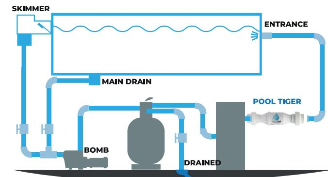
If the return line is too short to install the PoolTiger® inline, a bypass must be performed. Pool Tiger® can be installed horizontally, vertically or diagonally.
