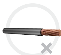
Damaged or cut-off individual wires
