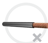
Excessively twisted individual wires
