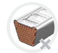
Formation of cracks at the sides. Sides split open
